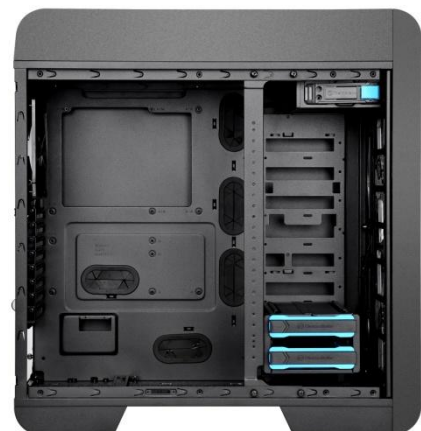
2 Bay cage installation
